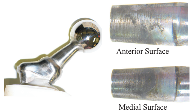
Figure 10 — Preliminary modular neck design with CoCr monoblock head/neck and Ti-6Al-4V stem and post-accelerated corrosion fatigue test surface condition of the CoCr neck taper.
