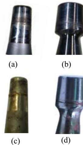
Figure 5 — Laboratory taper observations (a,b) representing accelerated corrosion fatigue test that most closely replicated the upper board of clinical observations (c,d) of the Ti-6Al-4V 6 degree and 12/14 head/stem tapers.
